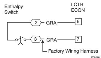
Fig. 48 - Enthalpy Switch (HH57AC077) Connections
